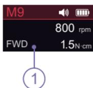
Before start the motor, check the operation mode ( ① ) is correct, otherwise press **S** once during standby state, press **-** or **+** to change.
